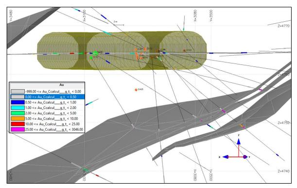
Figure 10-1 Underground drilling (section view)
