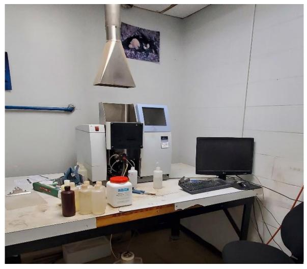
Figure 12-3 Atomic absorption instruments
