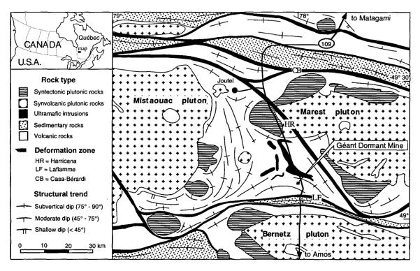
Figure 7-1 Simplified geological map of the mine district showing the location of the Sleeping Giant gold deposit close to the central part of a triple junction of structural trends. Map modified from Hocq (1990) and Chown et al. (1992).
