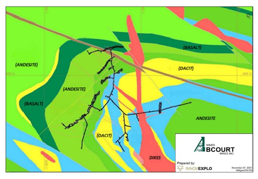
Figure 7-5 Plan view of level 665 showing development (note the angular relationship of the development with respect to geological contacts)
