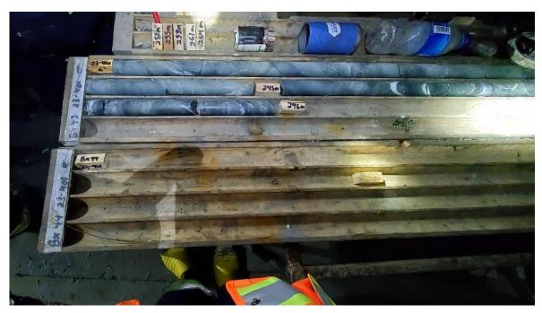
Figure 10-4 Wooden blocks placed every 3 metres by drill helper
