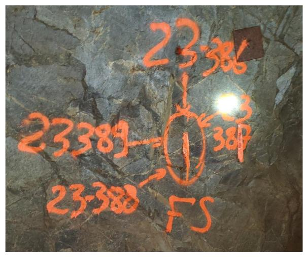
Figure 10-3 Front-sight for underground drill hole collar surveying
